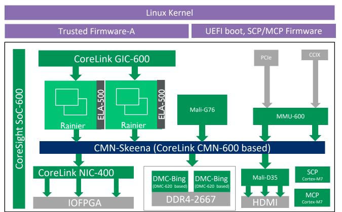
Supporting Arm system IP: GIC-600 (Generic Interrupt Controller), MMU-600 (IO MMU), Dynamic Memory Controller derived from DMC-620, SoC-600 (SoC Debug and Trace), Coherent Mesh Network derived from CMN-600, NIC-400 (Non-coherent interconnect)
