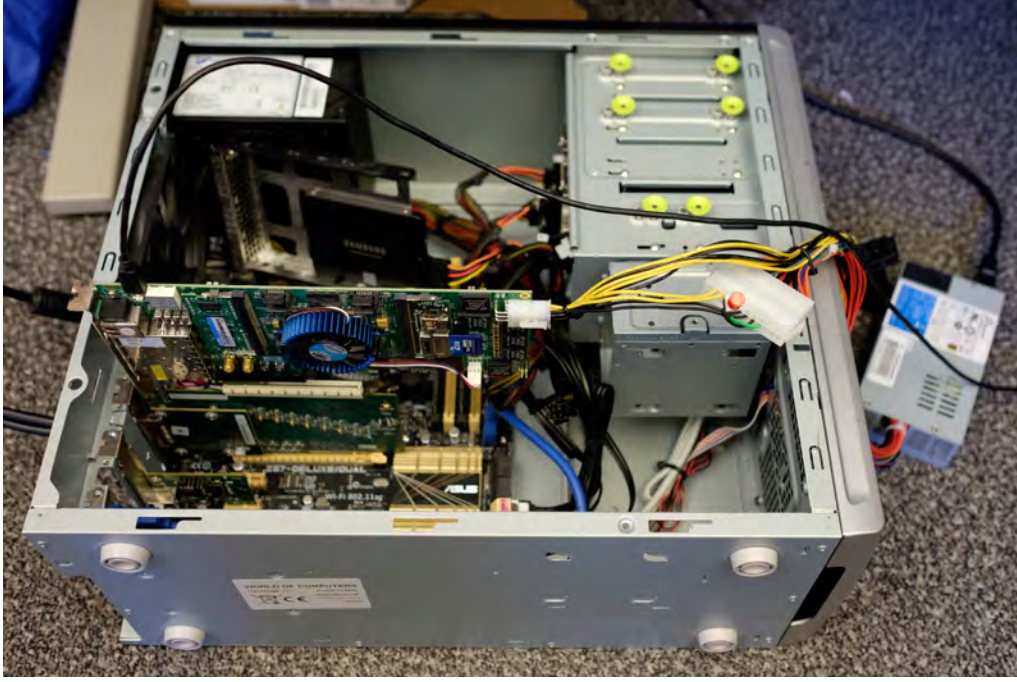
Figure 4.2: Photograph of Windows, Linux and FreeBSD experimental setup. This includes the FPGA in the riser for the PCIe analyser. The OS was varied on the victim by replacing the hard drive.
